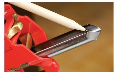
6. Wearing proper eye protection, grind the tool to chosen profile. Be careful not to roll the tool holder too far side to side as this lateral movement determines how far up the tool the cutting edge will go.
