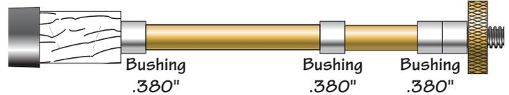
2. Advance a 60° revolving cone center into the dimpled end of the mandrel and tighten using light pressure. **Do Not** over tighten the tailstock or mandrel nut as this may cause the mandrel to flex resulting in off-center barrels.
