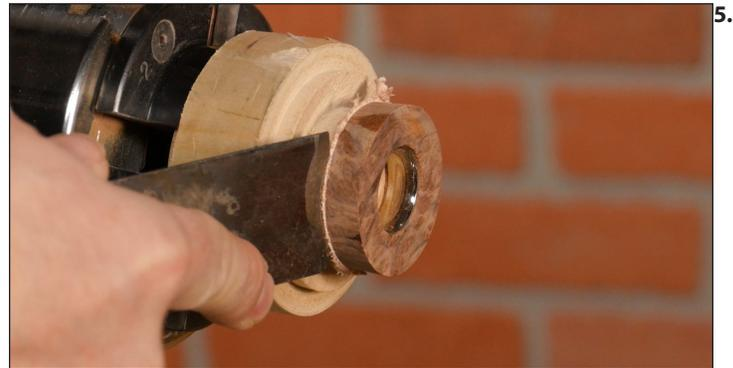
Lightly coat the inside of the ring blank with thick or flexible CA glue or Epoxy and insert the ring core. Wipe away any excess glue.
